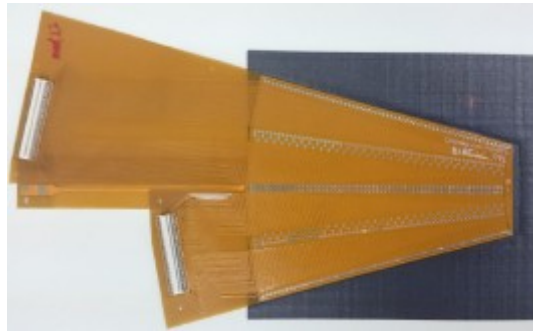
Fig. 3 A thin detector plane. The black part is the carbon fibre support, the silicon sensor is covered by the Kapton fan-out
