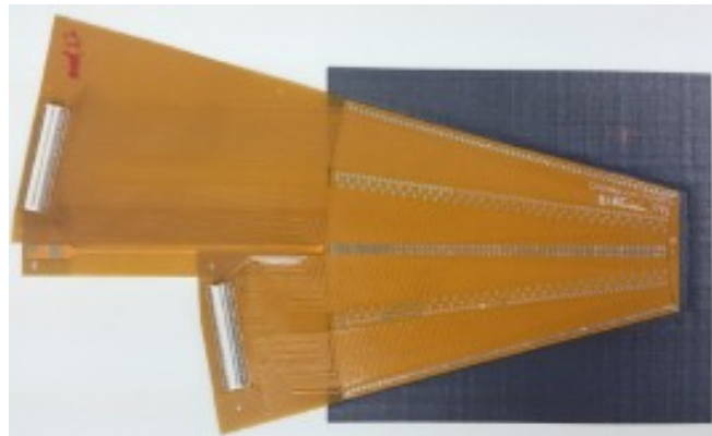
Fig. 3 A detector plane. The black part is the carbon fibre support, the silicon sensor is covered by the Kapton fan-out
