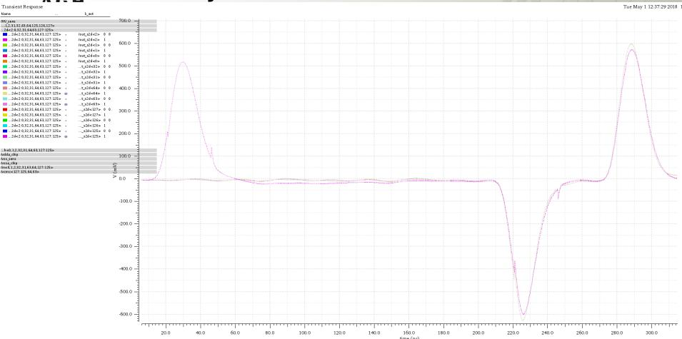
• First pulse injected externally, next two from Calibration
