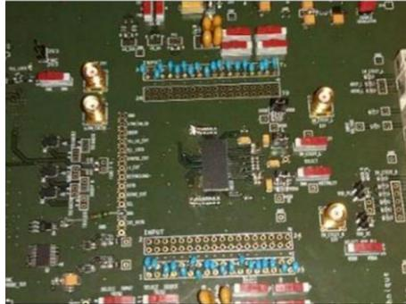
Figure 3.24: HGCROC V2 BGA testing board [13].
