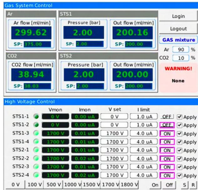
Figure 2.39: Screenshot of STS monitor desktop 1. Gas System Control (top) with gas flow and pressure monitor, and High Voltage Control (bottom) with supply high voltage and current for each part of STS [in courtesy of HADES collaboration].
