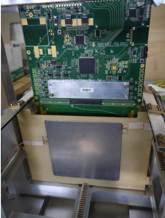
a) Photograph of readout board with silicon sensor mounted in supporting structure, preceded by the tungsten absorber layer
