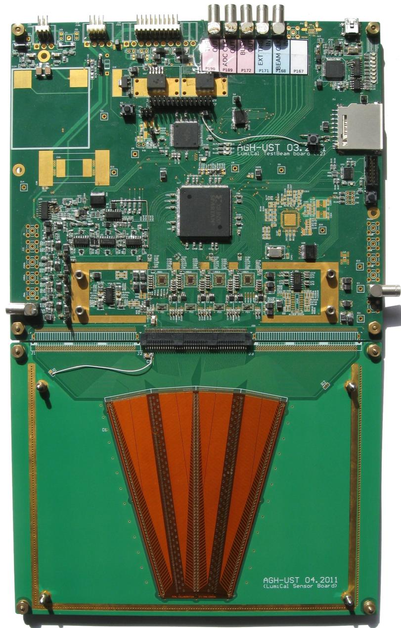
**Figure 1.23:** Photograph of the single layer *LumiCal* detector readout module.
