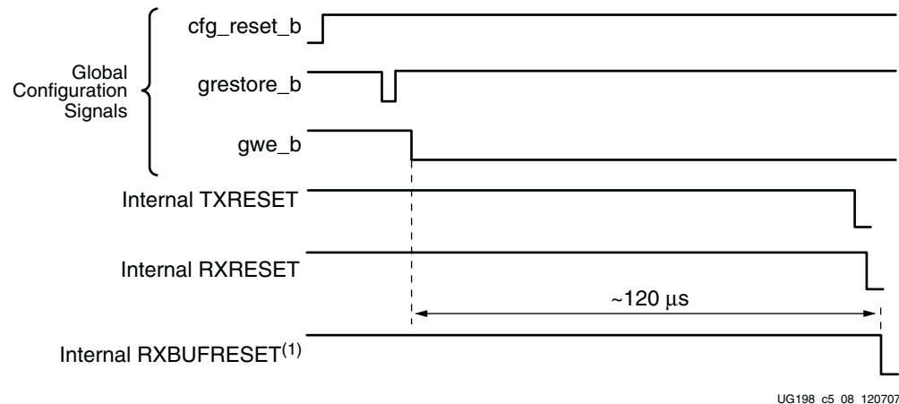
Figure 5-9: Reset Sequence Triggered by the GTXRESET Pulse
