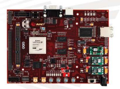
The Xilinx Virtex-5 FXT Evaluation Kit provides the necessary features for exploring PowerPC 440 based system architectures using the Xilinx Virtex-5 FXT FPGA family. This low cost evaluation platform is ideal for both software and FPGA designers needing an easy to use, entry level system for code development and debug, processor systems prototyping, and general FXT evaluation.
